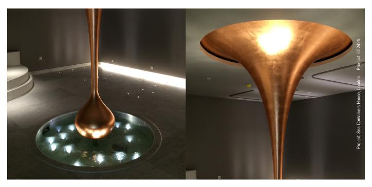
The LD242A has been designed specifically for permanent submersion applications. It is manufactured from high grade 316 stainless steel and anodised aluminium. The LED module is potted to prevent moisture ingress via the cable and the fitting is mechanically sealed. The bezel is polished and passivated for extra protection against chlorine or salt water.
